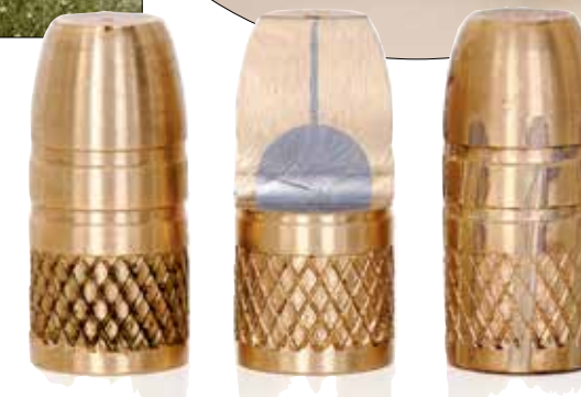
Big-time penetration: Belt Mountain's Big-Game Punch 300-grain .44 Mag load proved its mettle on live mesquite. A recovered bullet (inset, far right) showed only rifling marks after 11 inches of penetration.
