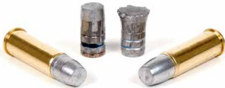
This recovered Garrett 330-grain Hammerhead (left) and Buffalo Bore 340-grain Hard Cast (right) were shot through 18 inches of soaked news-paper from an 18-inch rifle barrel.
